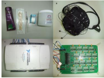
Figure 1 Experiment Equipment A : the electric gel ◦ B : 36-channel electrode cap ◦ C : NI USB-6212 analog to digital card ◦ D : 16-
